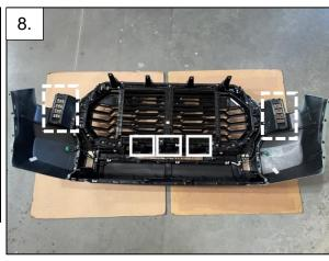
9. With snips, cut either side of the plastic piece spanning the opening in the two circled locations pictured on the front clip and discard.
